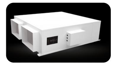
With flexible hanging options, an inbuilt drain tray, and an inbuilt controller offering both 0-10V DC Control for BMS and Manual 24V AC Control, this unit provides unparalleled versatility and control. The optional remote wall controller adds extra convenience, while spigots and hanging brackets ensure seamless integration into your ventilation infrastructure.
